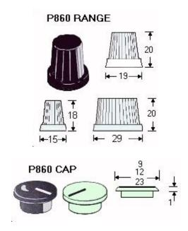
A matt textured black or brown ergonomically designed range of knobs with the choice of eleven different caps. The range covers 'Push On' or 'Grub Screw' fixings for our 4mm, 6mm and 6.35mm (1/4") Spindles. Also select a cap from our range of below.
