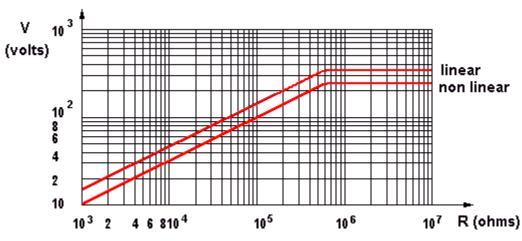
ECO, P16 maximum working voltage curve
