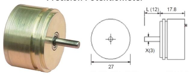
The servo potentiometers are constructed with a precision ball bearing system and long life flush bonded conductive track. The wipers have multiple fingers to achieve low contact resistance. The Resistive Element is Conductive Plastic (CP)
