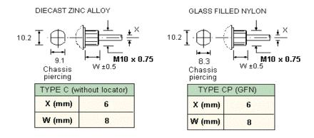
P16 Concentric Spindles and Tubes
