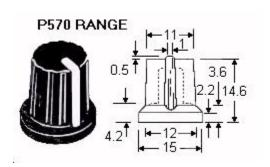
The spline knob features a matt black body with a choice of 9 different coloured pointers moulded into the body. The P570 is designed to push fit onto one of our 6mm Spline spindle.
