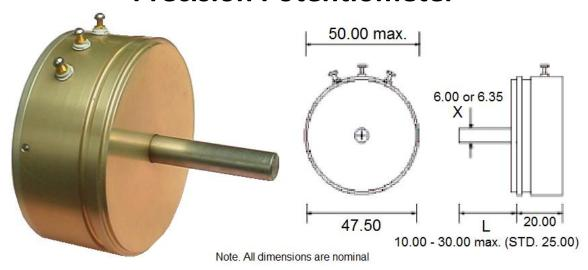
The servo potentiometers are constructed with a precision ball bearing system and long life flush bonded conductive track. The wipers have multiple fingers to achieve low contact resistance. The Resistive Element is Conductive Plastic (CP)
