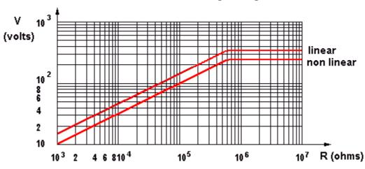
ECO, P16 maximum working voltage curve
