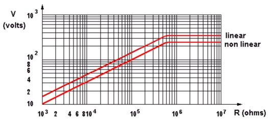
ECO, P16 maximum working voltage curve
