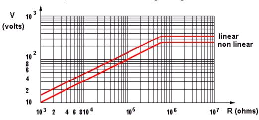
ECO, P16 maximum working voltage curve
