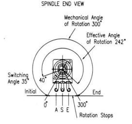
Total mechanical and effective electrical angles of rotation of potentiometers with rotary switch
