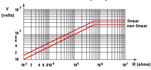
ECO, P16 maximum working voltage curve
