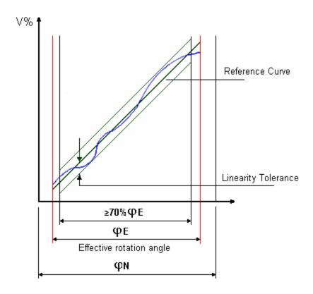
Matching Tolerance (For Tandem Stereo Potentiometers)
