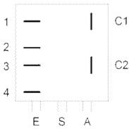
E 5 A Diagram as viewed on the rear of the switch module: (Potentiometer terminals at the bottom)
