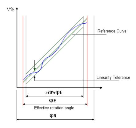
Matching Tolerance (For Tandem Stereo Potentiometers)
