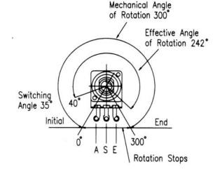
Total mechanical and effective electrical angles of rotation of potentiometers with rotary switch
