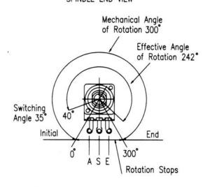
Total mechanical and effective electrical angles of rotation of potentiometers with rotary switch
